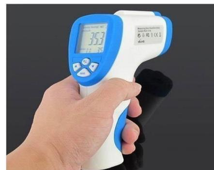
infrared (IR) energy onto a target body, and detects the energy, and displayed in the form of electrical signal which will be displayed in units of temperature.
